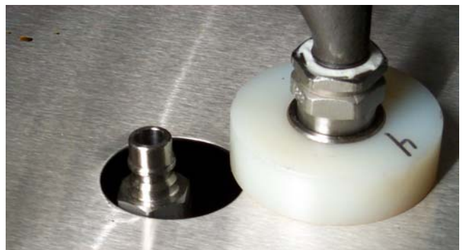
Pickup tube properly positioned in pan lid access hole.
